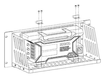
4. 固定仪器上部:将两个固定件压紧仪器上部,用 4 颗 M4 螺钉固定。 Fix the top of the instrument: fix the top of the instrument using two built-in fittings and four M4 screws.
