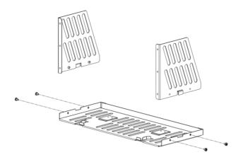
2. 安装机架前面板:将前面板用 6 颗 M4 螺钉固定在上一步装好的框架上。 Install the front panel of the rack mount kit: fix the front panel onto the frame installed in the previous step using six M4 screws.
