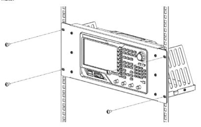
6. 安装后注意: 机架占 4U 高度,箭头所指的孔为机架的安装孔,注意对准安装。 Post-installation notice: the rack occupies a height of 4U. The holes pointed out by the arrows are installation holes. Note that they should be aligned with during installation.
