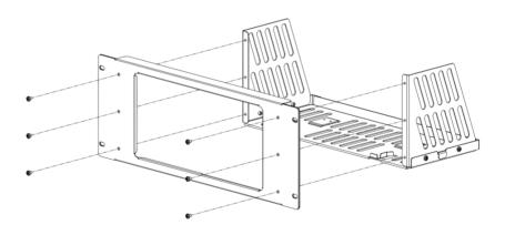
3. 固定仪器脚部:用两个压脚将仪器紧扣在底板上,用 4 颗 M4 螺钉将其固定。 Fix the bottom of the instrument: fix the instrument onto the support board using two pressure feet and four M4 screws.
